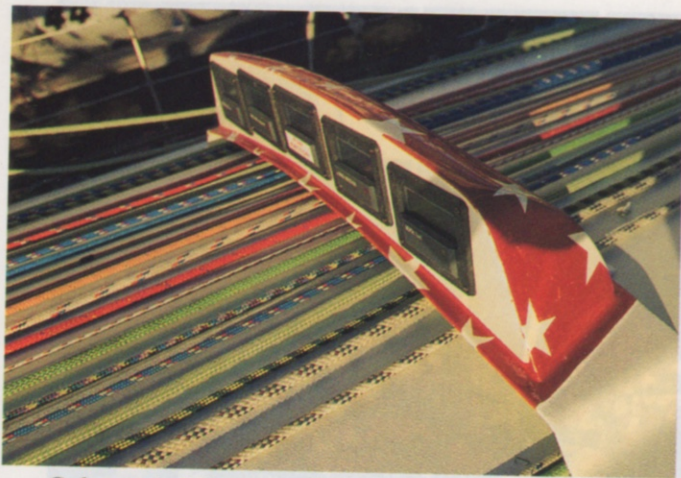
Color-coded lines that allow Steve Pettengill to raise, lower or reef his sails lead back to the boat's cockpit.
